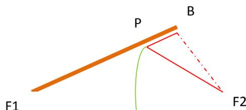
Note que de facto:  $\overline{PF_1} = L - \overline{PB}$ ,  $\overline{PF_2} = L - d - \overline{PB}$  e, portanto,  $\overline{PF_1} - \overline{PF_2} = d$
